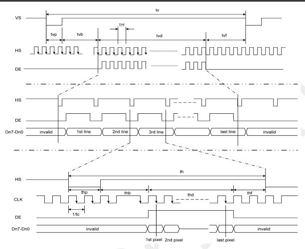
Serial RGB input timing requirement
