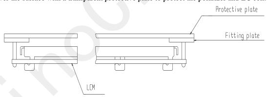
(2) When assembling the LCM into other equipment, the spacer to the bit between the LCM and the fitting plate should have enough height to avoid causing stress to the module surface, refer to the individual specifications for measurements. The measurement tolerance should be  $\pm 0.1$ mm.
