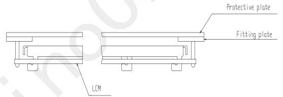
(2) When assembling the LCM into other equipment, the spacer to the bit between the LCM and the fitting plate should have enough height to avoid causing stress to the module surface, refer to the individual specifications for measurements. The measurement tolerance should be  $\pm 0.1$ mm.
