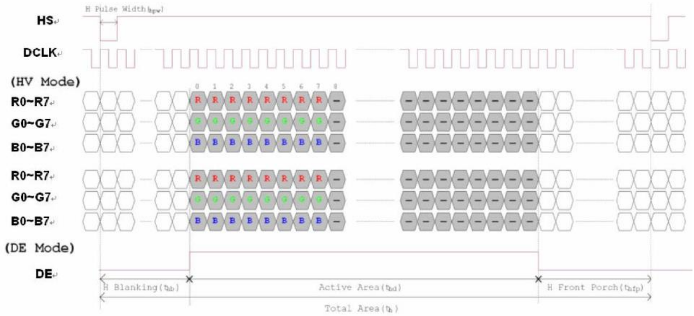
Figure 3. 1 Horizontal input timing diagram.
